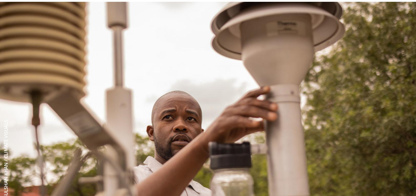
*A technician in Johannesburg checks and cleans the inlets of the ambient air quality monitoring station managed by South African Weather Services. This system measures traffic pollution and mine dump dust.*
